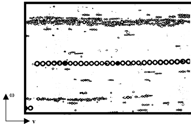
Figure 17. Alignment and segregation effects in suspensions of spheres suspended in a viscoelastic polyacrylamide solution displaying a pronounced alignment and segregation according to particle size when observed in the v - \omega plane (adapted from Giesekus (1978)). The arrow indicates the flow direction.
